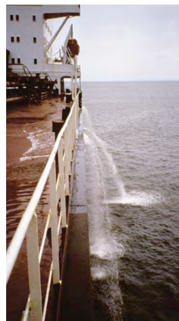
Flow-through ballast water exchange.
