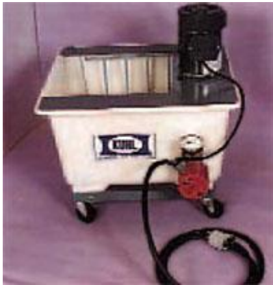
The KF Model is a low capacity immersion egg washer. [Photo courtesy of Kuhl Corporation.]
